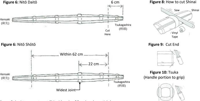
Figure 8 depicts a way to cut Shinai (made of four bamboo sticks).
