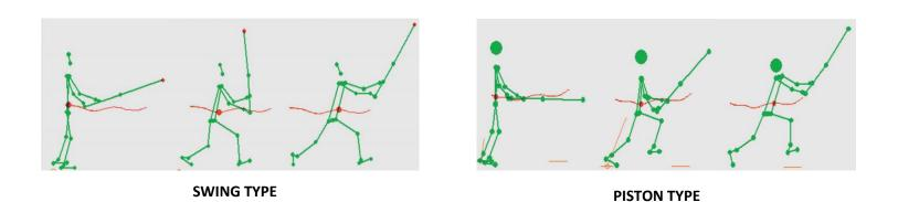
Swing type has the height position 83.47 cm from the floor at starting (Kamaye), 76.52 cm minimum and 80.75 cm maximum. Piston type has 89.5 cm at starting, 82.97 cm minimum and 89.34 cm maximum. Swing type falls 6.95 cm and rises 4.23 cm when strike. Whereas, Piston type falls 6.53 cm and rises 6.37 cm when strike. It was noted that Swing type has 6.95 - 6.53 = 0.42 cm more fall, and Piston type has 6.37 - 4.23 = 2.14 cm more rise.
